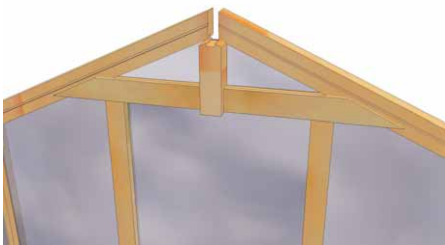
Rear Wall shown with Rafters, King Stud and Gable Support Frame configured correctly.
